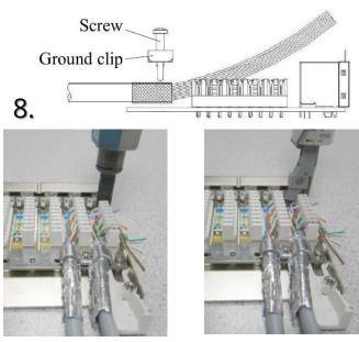
Install the wires into the IDC blocks according to the wiring position 568A/568B with 110/Krone punch down tool.
