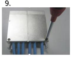
Put the rear cover into place and lock it into position by fastening the screw.
