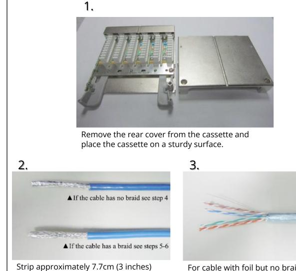
For cable with foil but no braid: Fold the foil shield back over the jacket of the cable.
