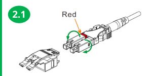
Rotate each ferrule 180 degrees so that the grey dots face to the bottom
