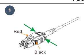
Press both sides to unlock the transparent clip
