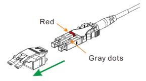
Pull the clip towards connectors end face and remove it completely
